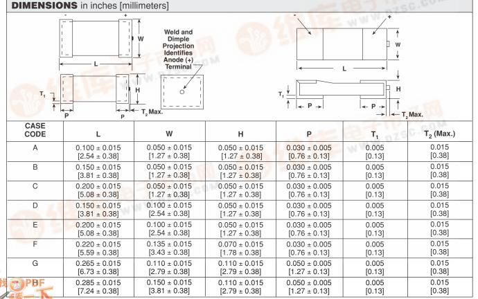
Note: When solder coated terminations are required, add .015" [0.38mm] to termination dimension tolerances.
