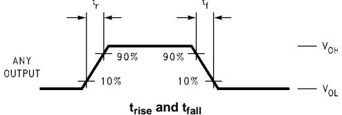
FIGURE 2. Waveforms
