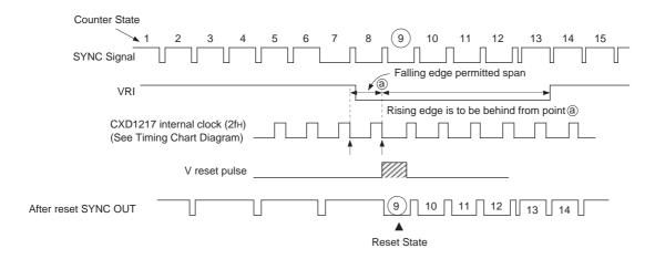
Since the falling edge point in the diagram above (marked with ↑) is the boundary of reset, if the falling edge of the VRI input traverses that point, it causes 1/2H deviation to the reset state.
