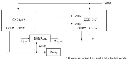
By varying the Delay and Shift Reg. of the above diagram, any phases of OHD2 and OVD2 can be provided against the respective OHD1 and OVD1.
