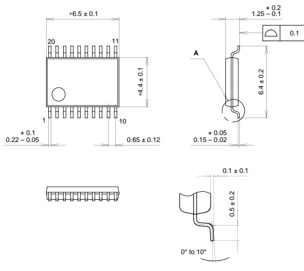
NOTE: Dimension "\*" does not include mold protrusion.
