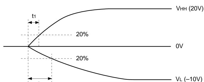
$t_2 \geq t_1 \geq 10\text{msec}$
