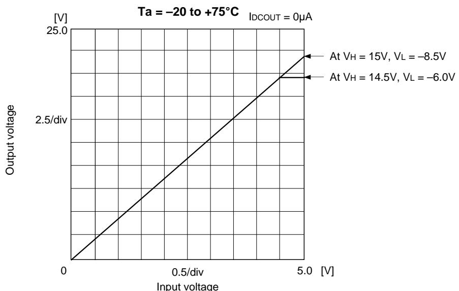
**Note)** Operating amplifier maximum output voltage is restricted as shown in the formula below depending on supply voltage setting of V<sub>H</sub> and V<sub>L</sub>.
