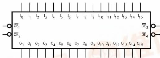
74VCXH16244 Low Voltage 16-Bit Buffer/Line Driver with Bushold
