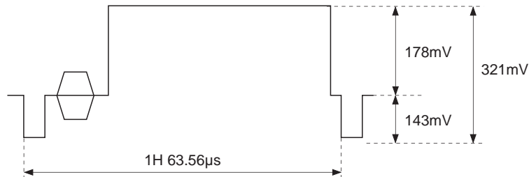
IN pin input waveform is the inverted waveform in the figure above
