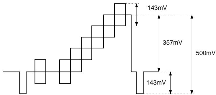
10. Input the 5-step staircase wave only for the luminance signal shown in the figure below, and measure the Y-OUT luminance level (Y) and SYNC level (S).
