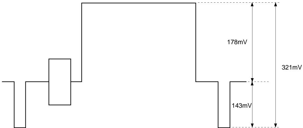
7. Measure the internal clock component (4fsc: 14.31818MHz component) when no signals are input.
