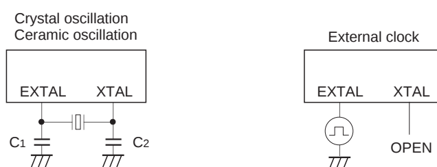
Fig. 2. Clock applying condition
