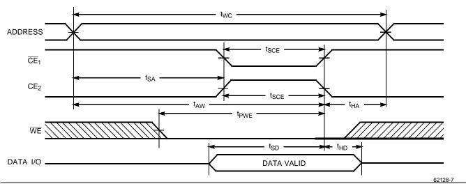
Write Cycle No. 2 ( $\overline{\text{WE}}$  Controlled,  $\overline{\text{OE}}$  HIGH During Write) $^{[13,14]}$
