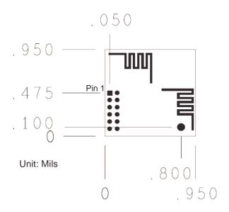
Figure 4-2. CYWM6935 Mechanical Drawing
