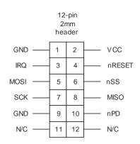
Figure 4-1. CYWM6935 Header Pin-out
