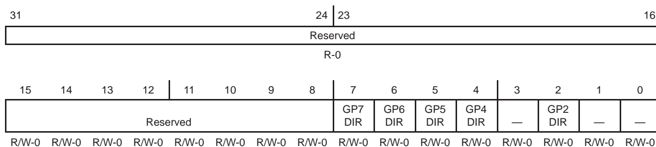
Figure 11. GPIO Direction Register (GPDIR) [Hex Address: 01B0 0004]
