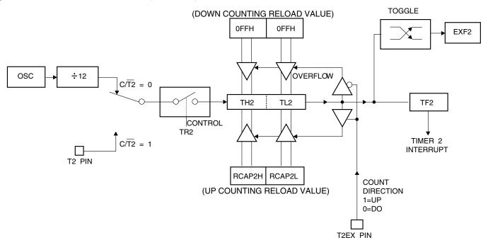
Figure 8. Timer 2 in Baud Rate Generator Mode
