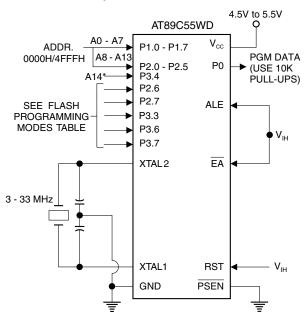
Note: \*Programming address line A14 (P3.4) is not the same as the external memory address line A14 (P2.6).
