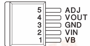
5-PIN TO-263 TD PACKAGE (TOP VIEW)
