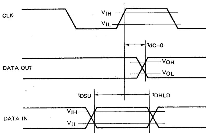
$t_{DC-0} : 2 \mu s$  MAX. ( $R_L=33 k\Omega$ ,  $C_L=15 pF$ ) $t_{DSU} : 2 \mu s$  MIN. $t_{DHLD} : 2 \mu s$  MIN.**INPUT AND OUTPUT CIRCUITS FOR  $\mu$ PD1990AC****Input circuits**
