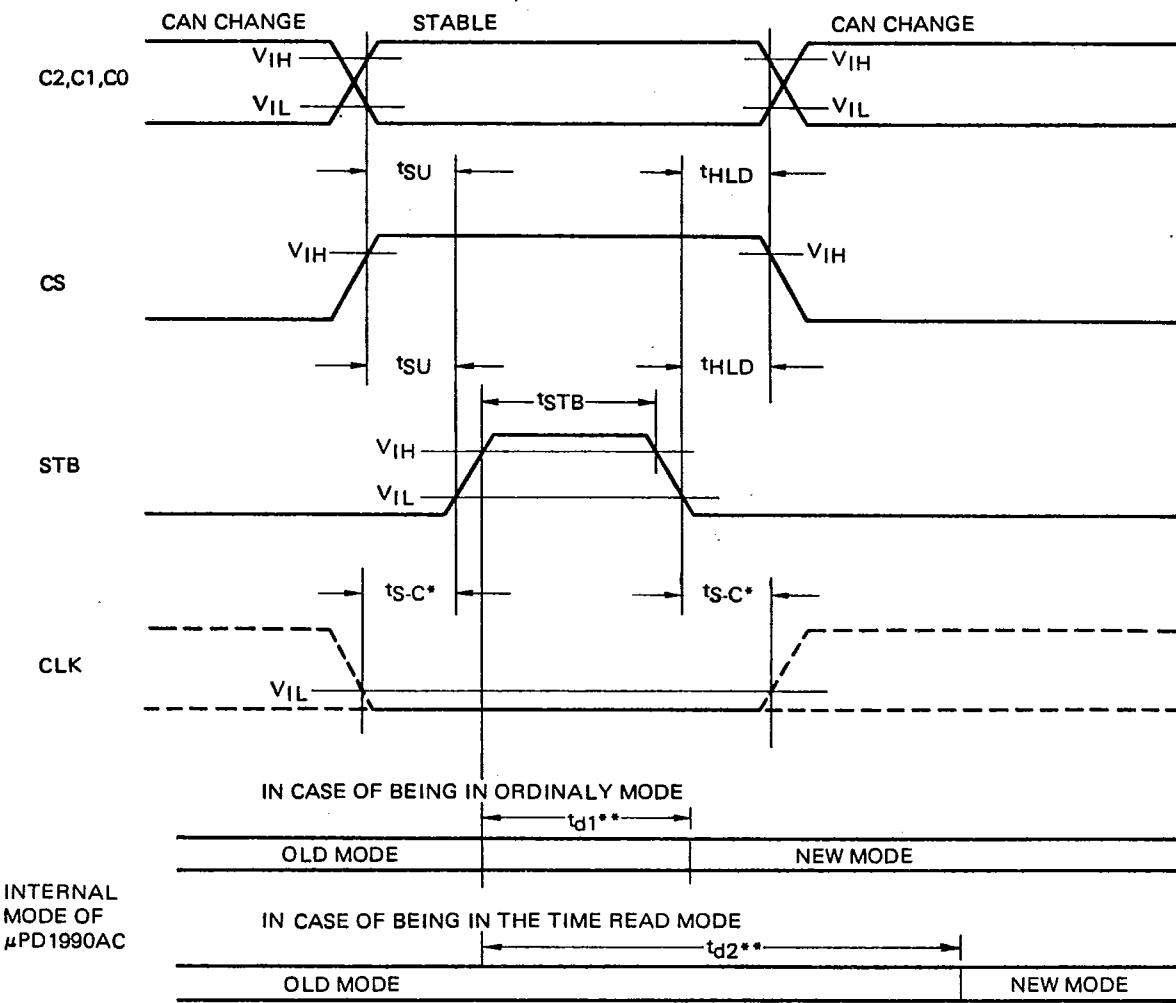
$t_{SU}$  = 2  $\mu$ s MIN. $t_{HLD}$  = 2  $\mu$ s MIN. $t_{STB}$  = 2  $\mu$ s MIN. $td_1$  = 4  $\mu$ s MAX. (In case of being in ordinary mode.) $td_2$  = 40  $\mu$ s MAX. (In case of being in the Time Read mode.) $t_{S-C^*}$  = 2  $\mu$ s MIN.
