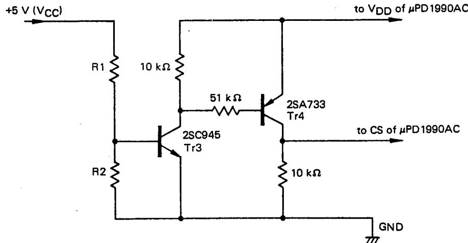
The Power Down of V<sub>CC</sub> line makes CS terminal inactive, with R1 and R2 resistors.
