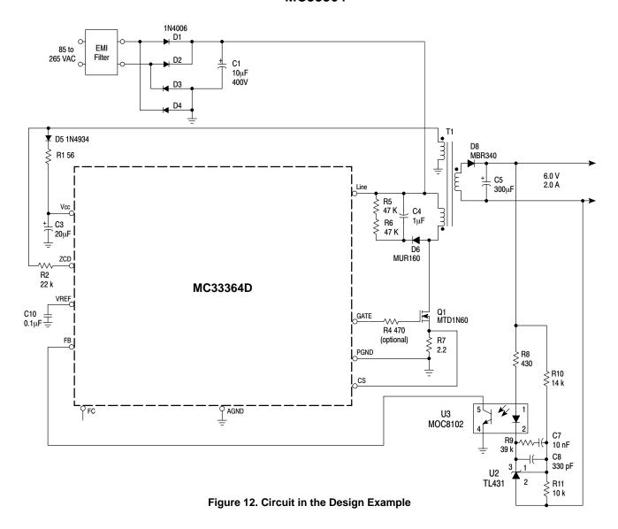
The described critical conduction mode flyback converter has the following performance and maximum ratings:
