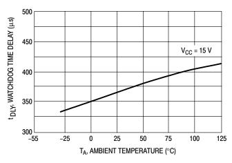
Figure 6. Watchdog Timer Delay versus Temperature
