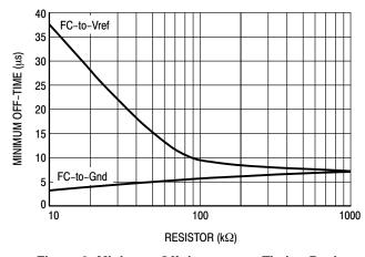
Figure 9. Minimum Off-time versus Timing Resistor on the FC Pin
