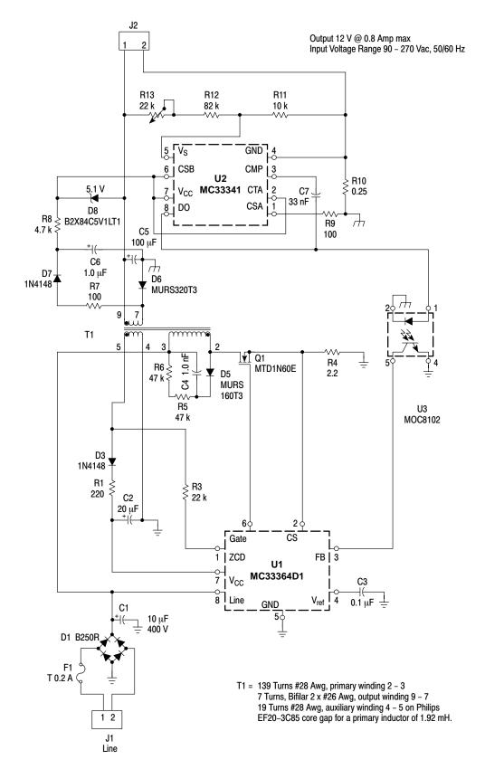
Figure 16. Universal Input Battery Charger
