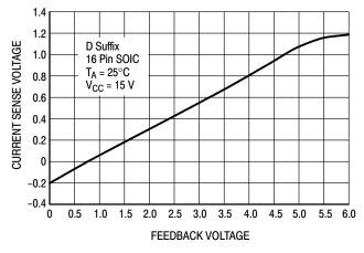
Figure 10. Feedback Voltage versus Current Sense Voltage
