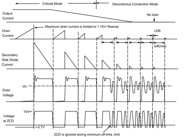
**Figure 4. Timing Diagram in Normal Condition**
