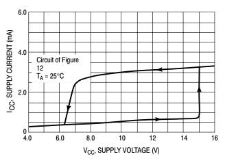
Figure 7. Supply Current versus Supply Voltage
