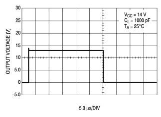
Figure 5. Drive Output Waveform
