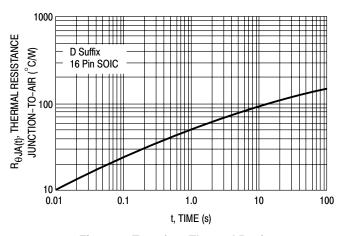
Figure 8. Transient Thermal Resistance
