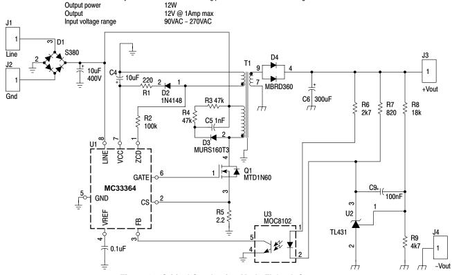
Figure 13. Critical Conduction Mode Flyback Converter
