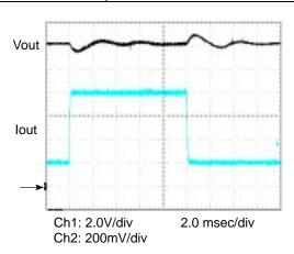
Figure 15. Load Regulation 240V
