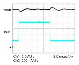
Figure 14. Load Regulation 120V
