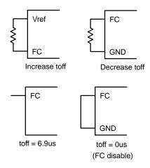
Figure 11. Frequency Clamp Setting
