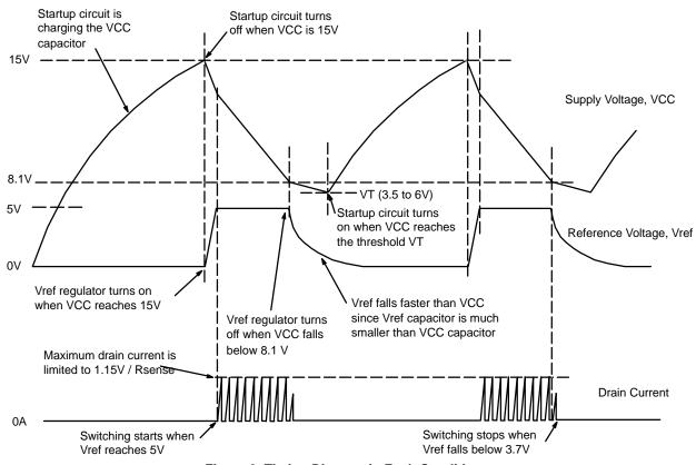
Figure 3. Timing Diagram in Fault Condition
