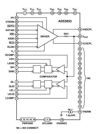
sensor is a current sink that is proportional to absolute temperature. The gain is trimmed to a nominal value of 1.0  $\mu A/K$ . As an example, the output current can be sensed by using a 10  $k\Omega$  resistor connected from +10 V to the THERM (IOUT) pin. A voltage drop across the resistor will be developed that equals:  $10K\times 1~\mu A/K=10~mV/K=2.98~V$  at room temperature.
