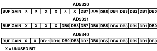
Figure 31. GAIN and BUF Data on a 16-Bit Bus
