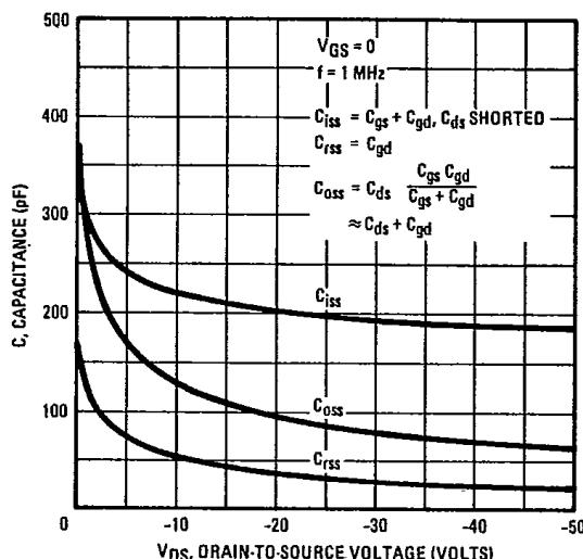
Fig. 9 – Typical Capacitance Vs. Drain-to-Source Voltage
