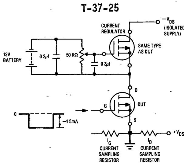
Fig. 17 — Gate Charge Test Circuit
