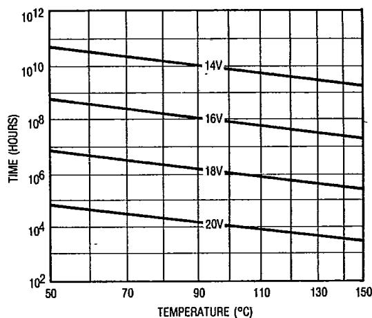
\*Fig. 18 — Typical Time to Accumulated 1% Gate Failure
