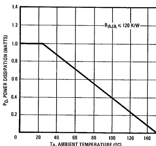
Fig. 13 – Power Vs. Temperature Derating Curve
