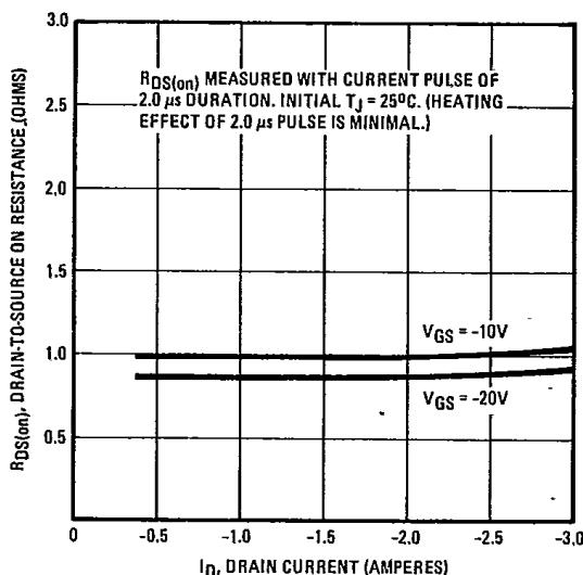
Fig. 11 – Typical On-Resistance Vs. Drain Current
