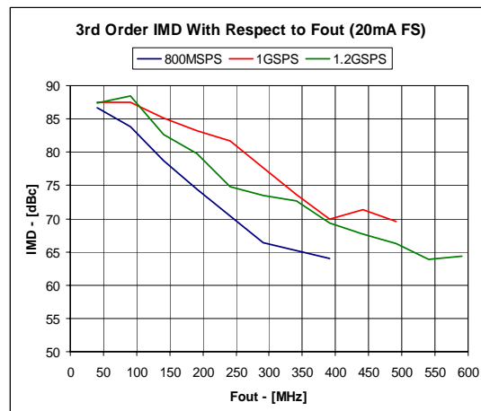
Figure 10. AD9736, 3 rd Order IMD vs. Fout and Sample Rate
