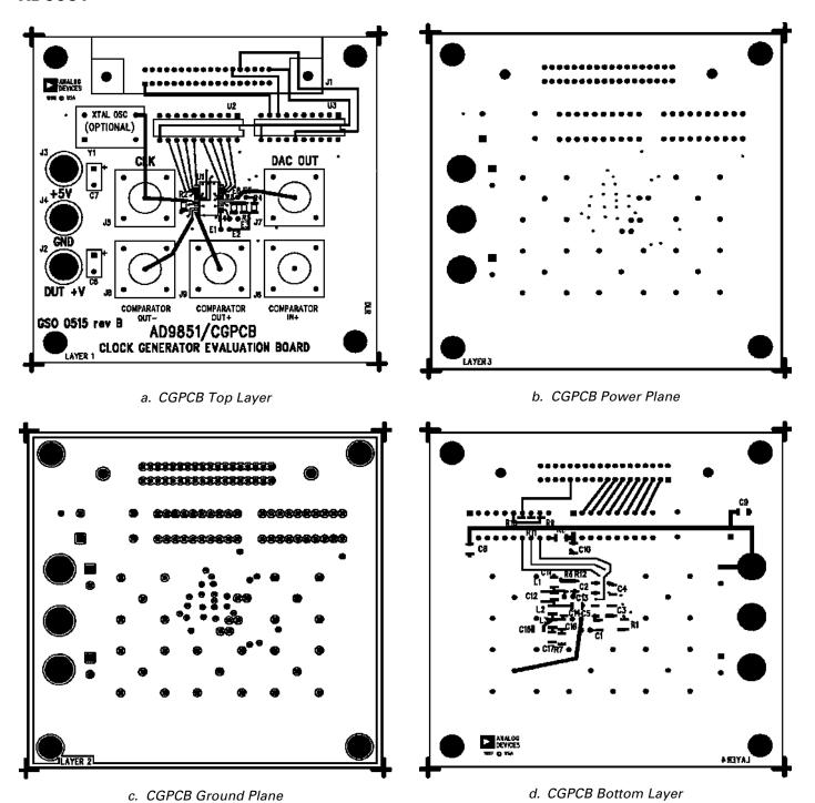
Figure 25. CGPCB Evaluation Board Four-Layer PCB Layout Patterns
