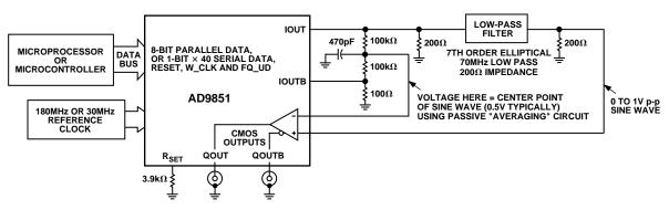
Figure 2. Basic Clock Generator Configuration
