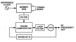
Figure 4. Frequency/Phase-Agile Reference for PLL
