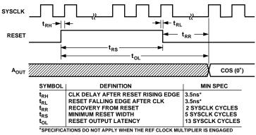
Figure 14. Master Reset Timing Sequence
