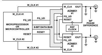
Figure 7. Application Showing Synchronization of Two AD9851 DDSs to Form a Quadrature Oscillator
