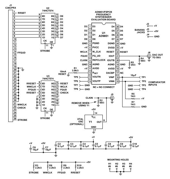
Figure 22. FSPCB Electrical Schematic
