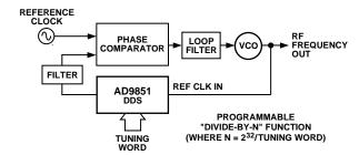
Figure 5. Digitally-Programmable "Divide-by-N" Function in PLL
