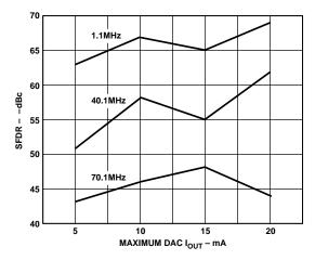
Figure 42. Effect of DAC maximum output current on wideband (0 to 72 MHz) SFDR at three representative DAC output frequencies: 1.1 MHz, 40.1 MHz and 70.1 MHz.  $V_S = +5 V$ , 180 MHz system clock (6× REFCLK Multiplier disabled). Currents are set using appropriate values of  $R_{SET}$ .
