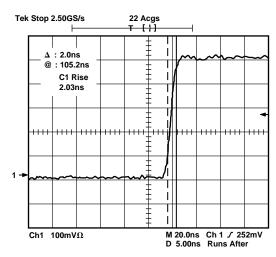
Figure 38. Comparator Rise Time, 15 pF Load
