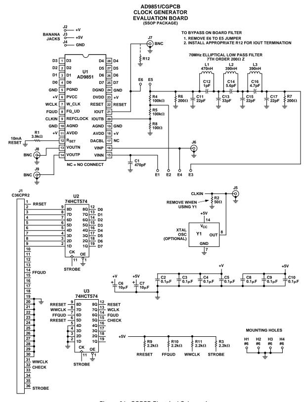
Figure 24. CGPCB Electrical Schematic
