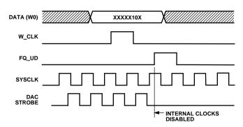
Figure 15. Parallel-Load Power-Down Sequence/Internal Operation
