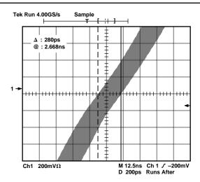
Figure 34. Typical CMOS comparator p-p output jitter with the AD9851 configured as a clock generator, DDS  $f_{OUT}$  = 70.1 MHz,  $V_S$  = +5 V, system clock = 180 MHz, 70 MHz LPF. Graph details the center portion of a rising edge with scope in delayed trigger mode, 200 ps/div. Cursors show 280 ps p-p jitter.
