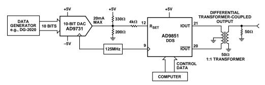
Figure 10. The AD9851 R<sub>SET</sub> Input Being Driven by an External DAC
