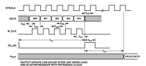
Figure 13. Parallel-Load Frequency/Phase Update Timing Sequence
