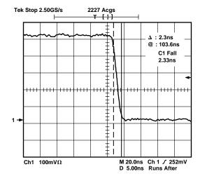
Figure 39. Comparator Fall Time, 15 pF Load
