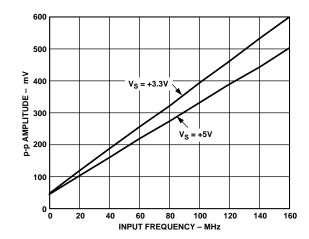
Figure 43. Minimum p-p input signal needed to toggle the AD9851 comparator output. Comparator input is a sine wave compared with a fixed voltage threshold. Use this data in addition to  $\sin(x)/x$  roll-off and any filter losses to determine if adequate signal is being presented to the AD9851 comparator.
