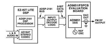
Figure 6. High Quality, All-Digital RF Frequency Modulation High quality, all digital RF frequency modulation generation
