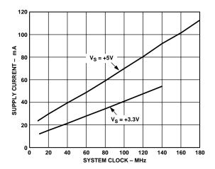
Figure 41. Supply current variation with system clock frequency.
