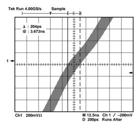
Figure 33. Typical CMOS comparator p-p output jitter with the AD9851 configured as a clock generator, DDS  $f_{OUT}$  = 40.1 MHz,  $V_S$  = +5 V, system clock = 180 MHz, 70 MHz LPF. Graph details the center portion of a rising edge with scope in delayed trigger mode, 200 ps/div. Cursors show 204 ps p-p jitter.
