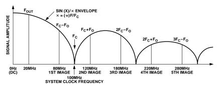
Figure 12. Output Spectrum of a Sampled Sin(X)/X Signal
