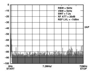
Figure 26. Wideband (dc to 72 MHz) output SFDR for a 1.1 MHz fundamental output signal. System clock = 180 MHz ( $6 \times REFCLK$  Multiplier engaged),  $V_S = +5 \text{ V}$ .
