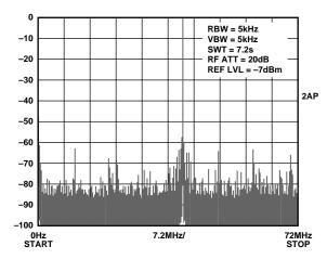
Figure 27. Wideband (dc to 72 MHz) output SFDR for a 40.1 MHz fundamental output signal. System clock = 180 MHz ( $6 \times REFCLK$  Multiplier engaged),  $V_S = +5 V$ .
