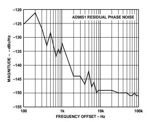
Figure 36. Output Residual Phase Noise (5.2 MHz  $A_{OUT}$ ),  $6 \times$  REFCLK Multiplier Disabled, System Clock = 180 MHz,
