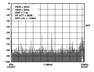
Figure 28. Wideband (dc to 72 MHz) output SFDR for a 70.1 MHz fundamental output signal. System clock = 180 MHz ( $6 \times REFCLK Multiplier engaged$ ),  $V_S = +5 V$ .
