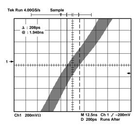
Figure 32. Typical CMOS comparator p-p output jitter with the AD9851 configured as a clock generator, DDS  $f_{OUT}$  = 10.1 MHz,  $V_S$  = +5 V, system clock = 180 MHz, 70 MHz LPF. Graph details the center portion of a rising edge with scope in delayed trigger mode, 200 ps/div. Cursors show 208 ps p-p jitter.
