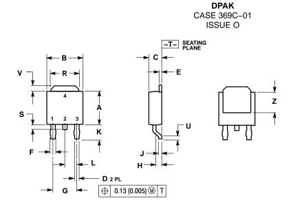
NOTES: 1. DIMENSIONING AND TOLERANCING PER ANSI Y14.5M, 1982. 2. CONTROLLING DIMENSION: INCH.
