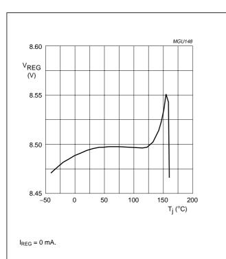
Fig.14 Output voltage as a function of the junction temperature.
