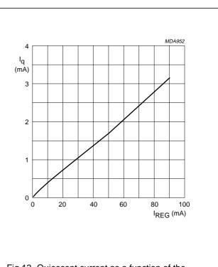
Fig.13 Quiescent current as a function of the output current.
