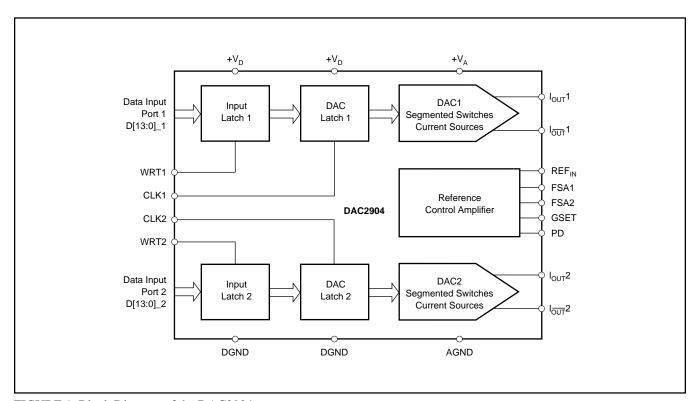
FIGURE 1. Block Diagram of the DAC2904.
