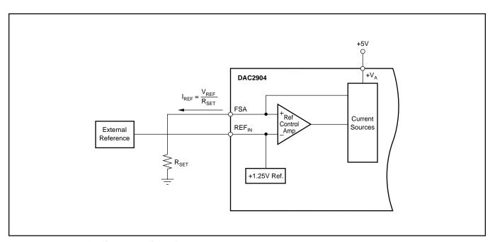
FIGURE 11. External Reference Configuration.
