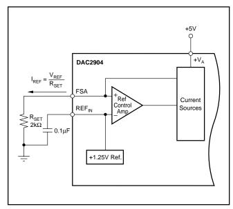
FIGURE 10. Internal Reference Configuration.
