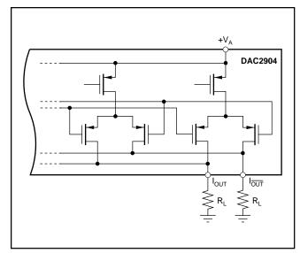
FIGURE 2. Equivalent Analog Output.
