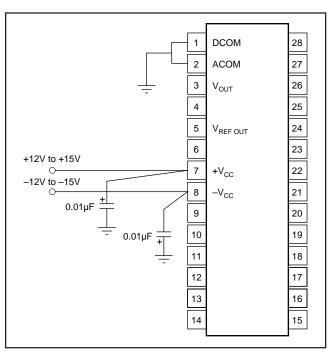
FIGURE 4. Power Supply Connections.
