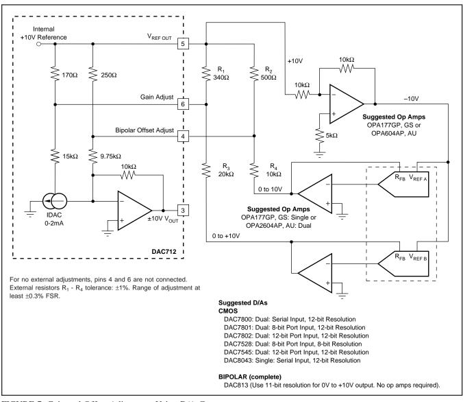
FIGURE 7. Gain and Offset Adjustment Using D/A Converters.
