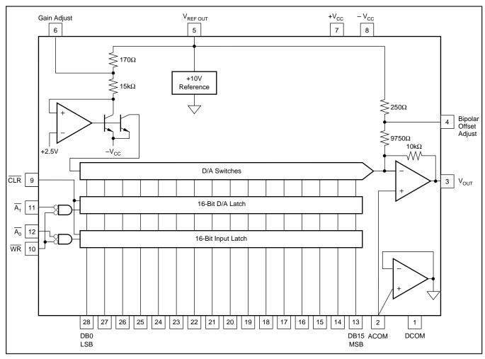
FIGURE 1. DAC712 Block Diagram.
