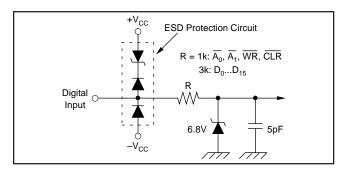
FIGURE 2. Equivalent Circuit of Digital Inputs.
