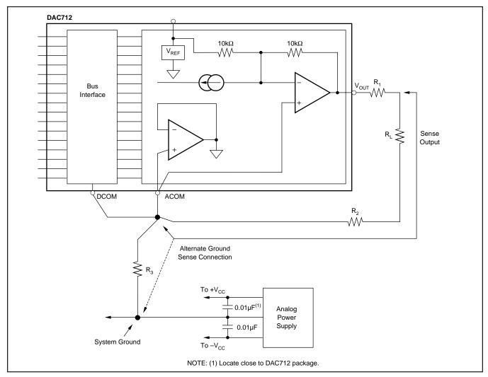
FIGURE 5. System Ground Considerations for High-Resolution D/A Converters.
