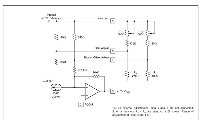
FIGURE 6. Manual Offset and Gain Adjust Circuits.
