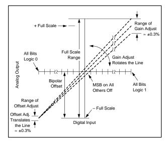
FIGURE 3. Relationship of Offset and Gain Adjustments.
