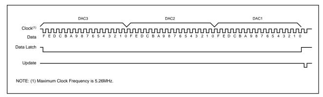
FIGURE 8b. Timing Diagram For Figure 8a.
