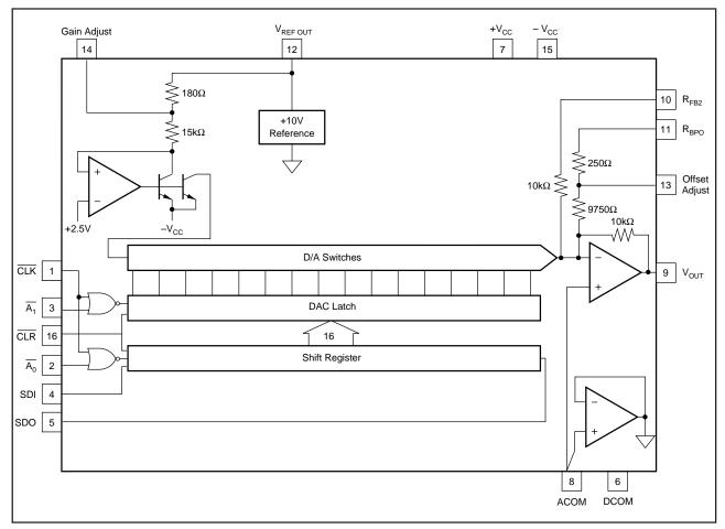
FIGURE 1. DAC714 Block Diagram.
