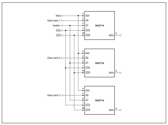
FIGURE 10a. Parallel Bus Connection.
