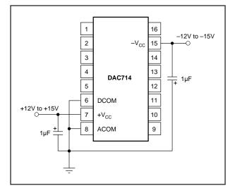
FIGURE 4. Power Supply Connections.
