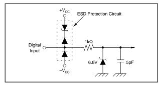
FIGURE 2. Equivalent Circuit of Digital Inputs.
