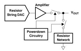
Figure 46. Output Stage During Power-Down
