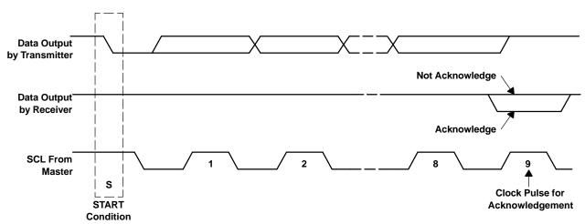
Figure 42. Acknowledge on the I<sup>2</sup>C Bus
