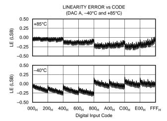
LINEARITY ERROR and DIFFERENTIAL LINEARITY ERROR vs CODE
