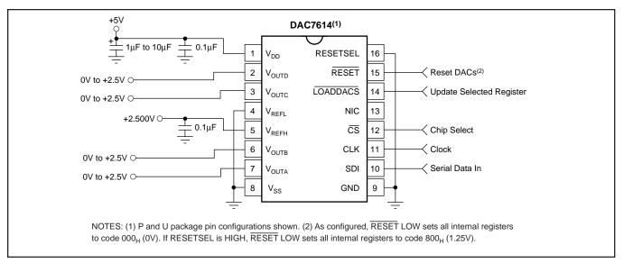
FIGURE 1. Basic Single-Supply Operation of the DAC7614.
