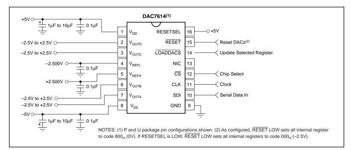
FIGURE 2. Basic Dual-Supply Operation of the DAC7614.
