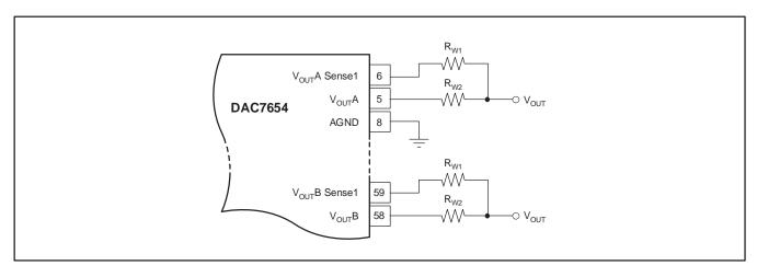
Figure 56. Analog Output Closed-Loop Configuration (1/2 DAC7654). Rw represents wiring resistances.
