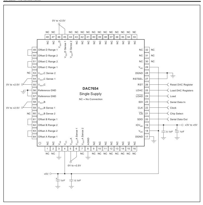
Figure 54. Basic Single-Supply Operation of the DAC7654
