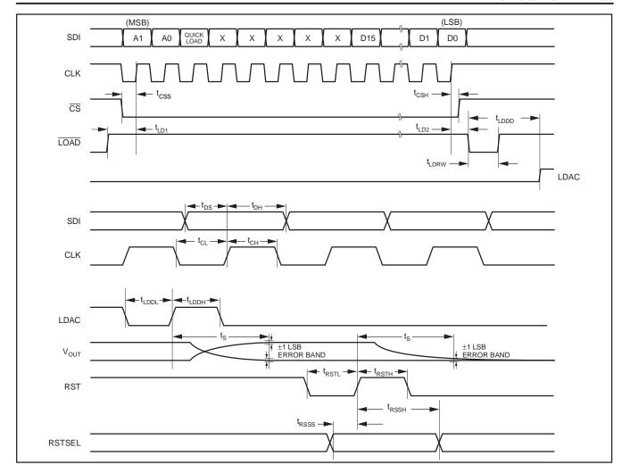
Figure 58. Digital Input and Output Timing
