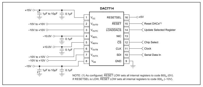
FIGURE 3. Basic Dual-Supply Operation of the DAC7714.
