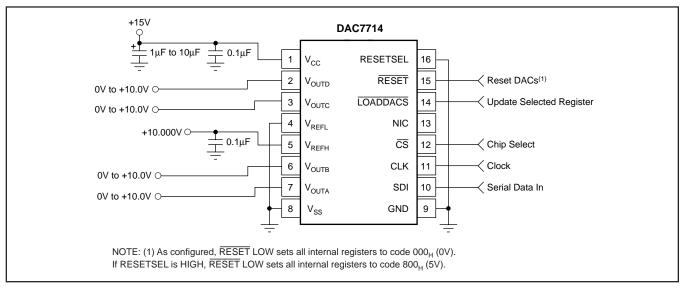
FIGURE 2. Basic Single-Supply Operation of the DAC7714.
