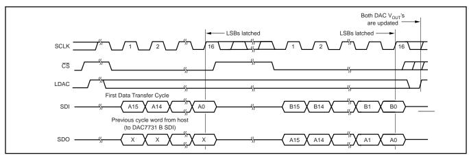
FIGURE 8. DAC7731 Daisy-Chain Timing for Figure 7.
