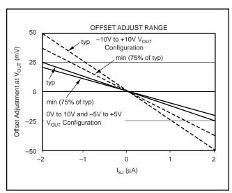
FIGURE 12. Offset Adjustment Transfer Characteristic.
