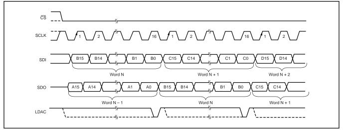
FIGURE 6. Continuous Transfer Control.
