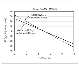
FIGURE 13. Internal Reference Adjustment Transfer Characteristic.
