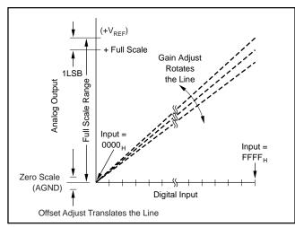
FIGURE 9. Relationship of Offset and Gain Adjustments for  $V_{OLIT} = 0V$  to +10V Output Configuration.
