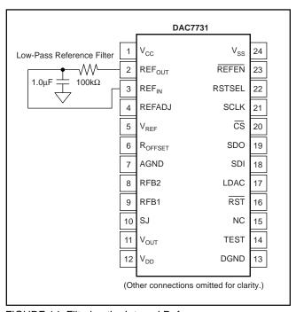
FIGURE 14. Filtering the Internal Reference.
