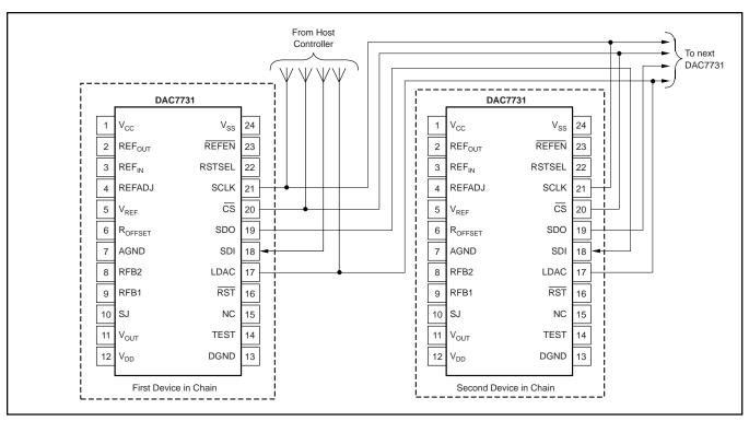
FIGURE 7. DAC7731 Daisy-Chain Schematic.
