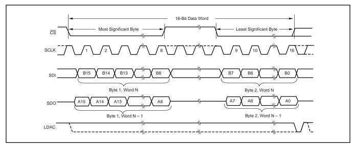
FIGURE 5. Byte-Wide Data Write Cycle.
