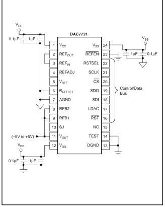
FIGURE 3. Basic Operation:  $V_{OUT} = -5V \text{ to } +5V.$
