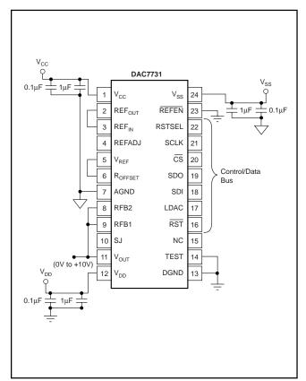
FIGURE 2. Basic Operation:  $V_{OUT} = 0V$  to +10V.
