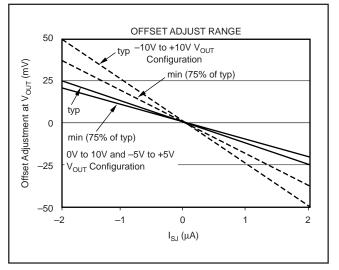
FIGURE 8. Offset Adjustment Transfer Characteristic.
