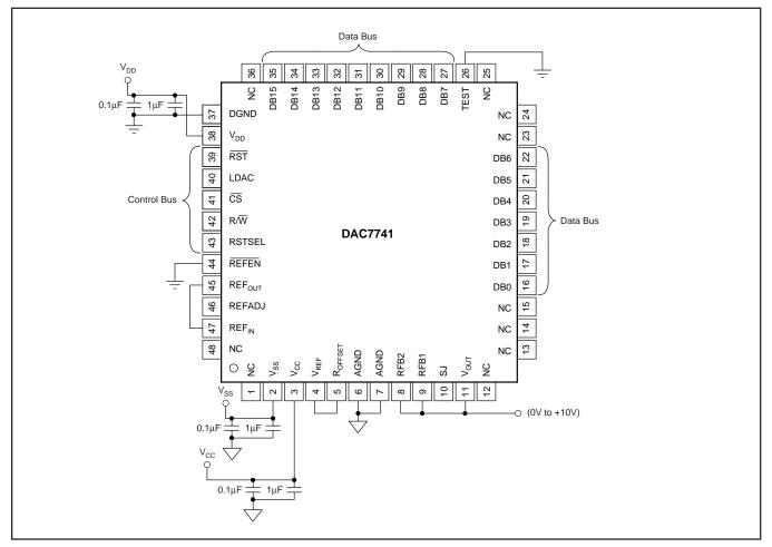
FIGURE 2. Basic Operation:  $V_{OUT} = 0$  to +10V.
