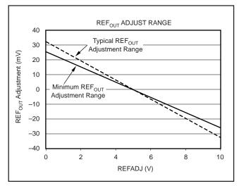
FIGURE 9. Internal Reference Adjustment Transfer Characteristic.
