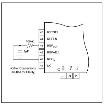
FIGURE 10. Internal Reference Filter.
