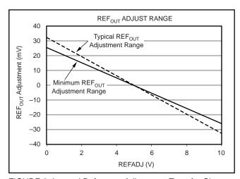
FIGURE 9. Internal Reference Adjustment Transfer Characteristic.
