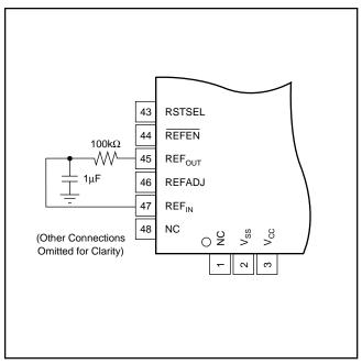
FIGURE 10. Internal Reference Filter.
