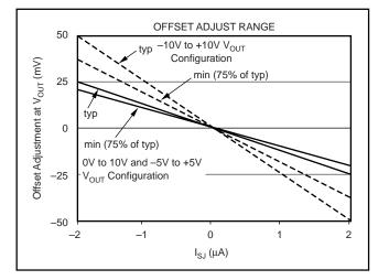
FIGURE 8. Offset Adjustment Transfer Characteristic.
