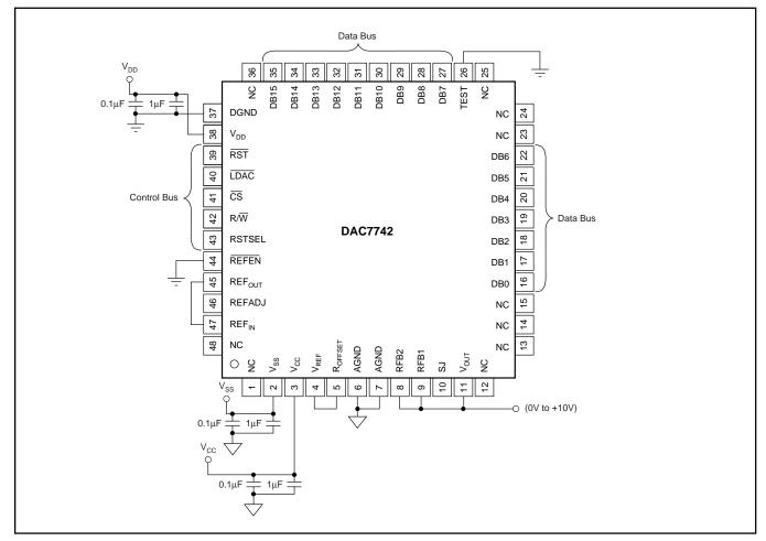
FIGURE 2. Basic Operation:  $V_{OUT} = 0V$  to +10V.
