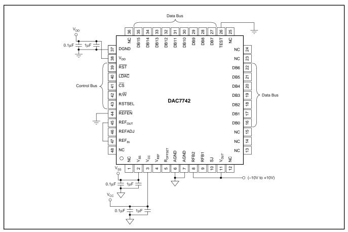
FIGURE 4. Basic Operation:  $V_{OUT} = -10V$  to +10V.
