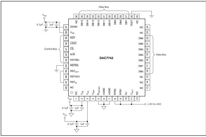
FIGURE 3. Basic Operation:  $V_{OUT} = -5V$  to +5V.
