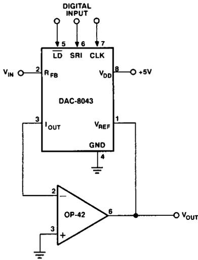
Figure 8. Analog/Digital Divider
