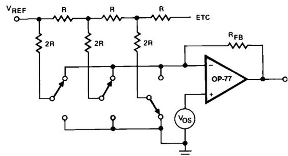
Figure 4. Simplified Circuit
