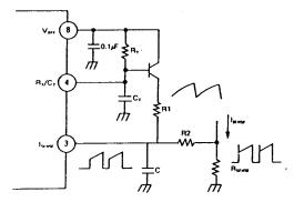
A fration of the oscillator ramp can be resistively summed with the current sense signal to provide slope compensation for coverters requiring duty cycle over 50%. Note that capacitor C, forms a filter with R2 to supress the leading edge switch spikes.
