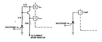
Shutdown of the DBL3842 can be accomplished by two methods; either raise pin3 above 1V or pull pin1 below a voltage two diodes drops above ground. Either method causes the output of the PWM comparator to be high(refer to
