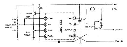
High peak currents associated with capacitive leads necessitate careful grounding techniques. Timing and bypass capacitors should be connected close to Pin 5 in a single point ground. The transistor and 5KQpotentiometer are used to sample the oscillator waveform and apply an adjustable ramp to Pin 3.
