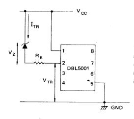
To operate the 5001 circuit from a DC 12V supply,  $R_E$  should be typically  $50K\Omega$ , This operation can also be used to reduce the effective value of the V  $_{CC(INI)}$ , by inserting a zener diode in series with  $R_E$ . Then, this initiating voltage V  $_{CC(INI)}$  is  $V_{IR} + V_Z + 10R_E$ .
