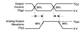
$\begin{array}{c} \text{VOLTAGE WAVEFORMS} \\ \textbf{t}_{\text{pd(s)}} \text{ TIMES} \end{array}$
