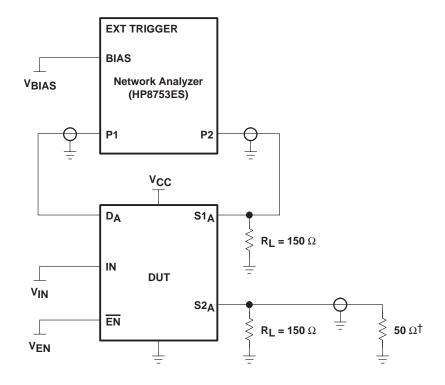
$^{\dagger}$  A 50- $\!\Omega$  termination resistor is needed for the network analyzer.
