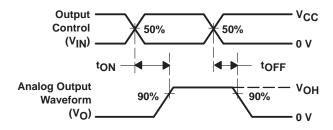
$\begin{tabular}{ll} VOLTAGE WAVEFORMS \\ ton AND toff TIMES \\ \end{tabular}$
