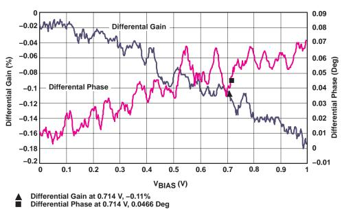
Figure 2. Differential Gain/Phase vs V<sub>BIAS</sub>
