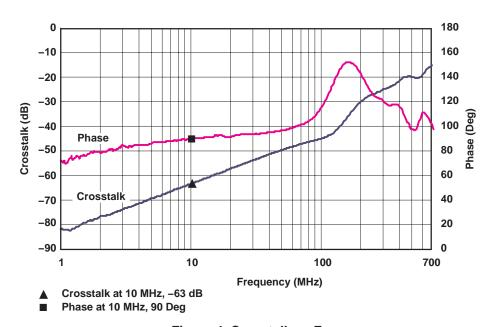
Figure 4. Crosstalk vs Frequency
