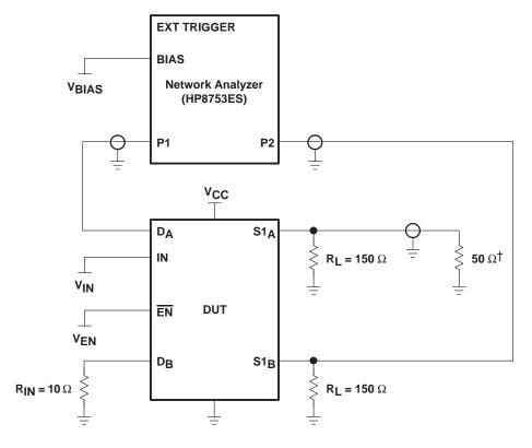
$^{\dagger}\,\text{A}$  50- $\!\Omega$  termination resistor is needed for the network analyzer.
