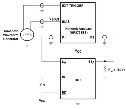
NOTE: For additional information on measurement method, refer to the TI application report, *Measuring Differential Gain and Phase*, literature number SLOA040.
