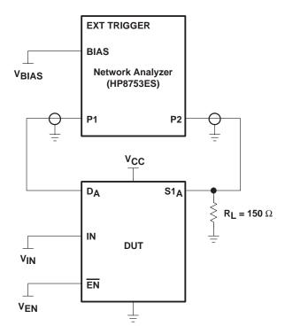
Figure 9. Test Circuit for Frequency Response (BW)
