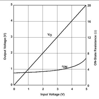
Figure 5. Output Voltage/ON-State Resistance vs Input Voltage
