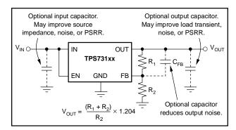
Figure 32. Typical Application Circuit for Adjustable-Voltage Versions
