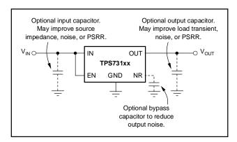
Figure 31. Typical Application Circuit for Fixed-Voltage Versions
