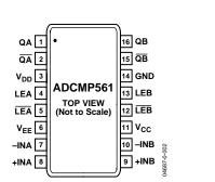
Figure 4. ADCMP561 16-Lead QSOP Pin Configuration
