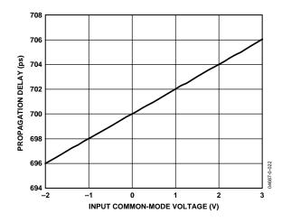
Figure 15. Propagation Delay vs. Common-Mode Voltage
