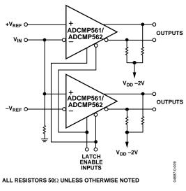
Figure 23. High Speed Window Comparator
