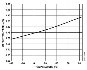
Figure 7. Input Offset Voltage vs. Temperature
