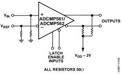
Figure 22. High Speed Sampling Circuits
