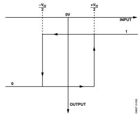
Figure 20. Comparator Hysteresis Transfer Function
