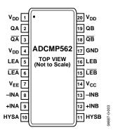
Figure 5. ADCMP562 20-Lead QSOP Pin Configuration
