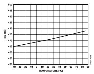
Figure 11. Fall Time vs. Temperature
