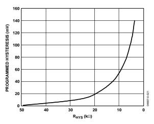
Figure 21. Comparator Hysteresis vs. R<sub>HYS</sub>
