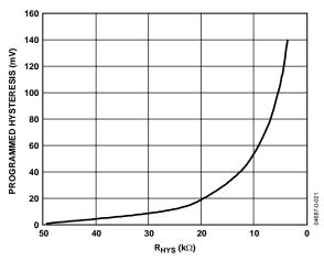
Figure 14. Comparator Hysteresis vs. R<sub>HYS</sub>
