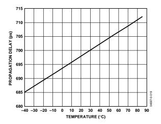
Figure 12. Propagation Delay vs. Temperature
