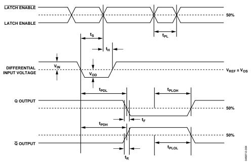
Figure 18. System Timing Diagram
