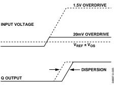
Figure 19. Propagation Delay Dispersion
