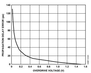
Figure 13. Propagation Delay vs. Overdrive Voltage
