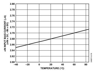
Figure 9. Input Bias Current vs. Temperature
