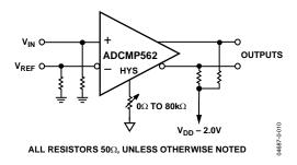
Figure 24. Adding Hysteresis Using the HYS Control Pin
