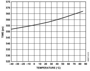
Figure 8. Rise Time vs. Temperature
