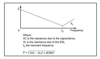
Figure 4. Capacitor Impedance vs Frequency
