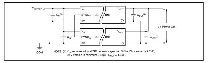
Figure 3. Connecting Multiple DCP01Bs in Parallel
