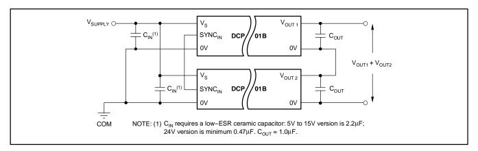
Figure 1. Connecting the DCP01B in Series
