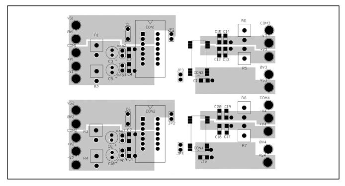
Figure 6. Example of PCB Layout, Non-component-Side View
