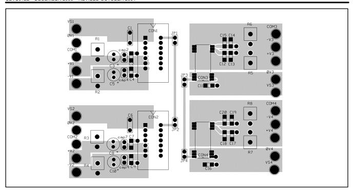
Figure 5. Example of PCB Layout, Component-Side View
