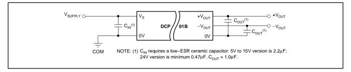
Figure 2. Connecting Dual Outputs in Series
