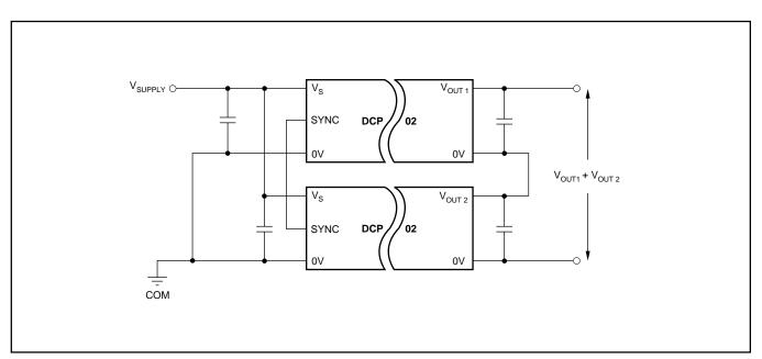
FIGURE 1. Connecting the DCP02 in Series.
