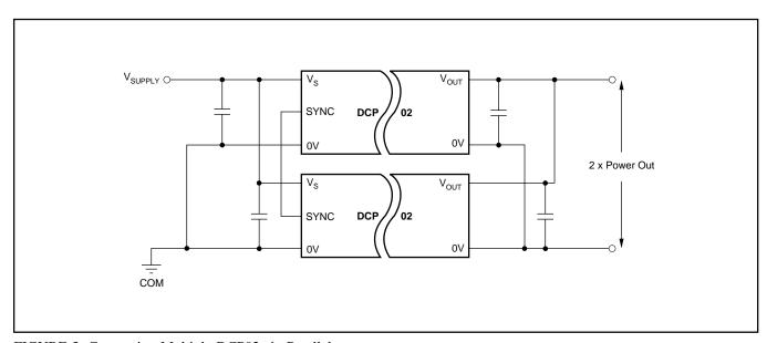
FIGURE 3. Connecting Multiple DCP02s in Parallel.
