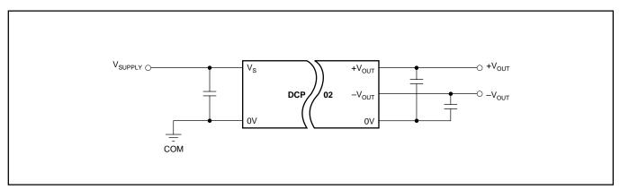
FIGURE 2. Connecting Dual Outputs in Series.
