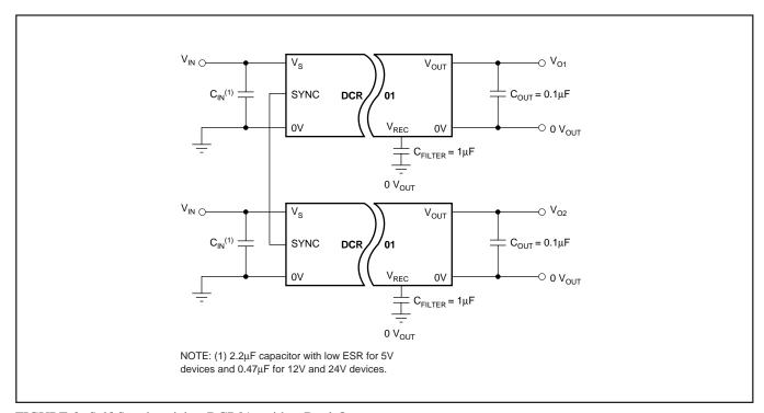
FIGURE 2. Self-Synchronizing DCR01s with a Dual Output.
