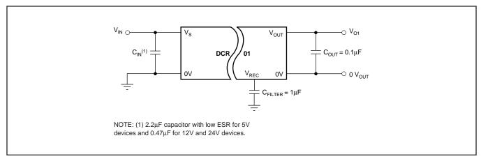
FIGURE 1. DCR01 with a Single Output.
