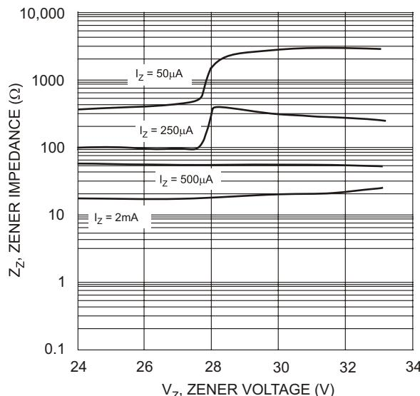
Fig. 14 Typical Zener Impedance Characteristics,
