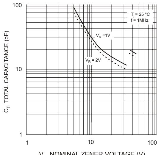
Fig. 20 Total Capacitance vs Nominal Zener Voltage
