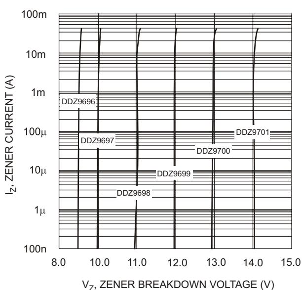
Fig. 5 Typical Reverse Characteristics, DDZ9696 - DDZ9701
