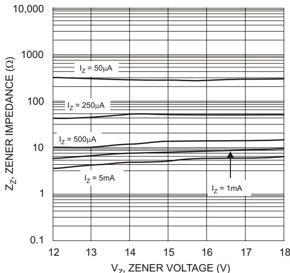
Fig. 12 Typical Zener Impedance Characteristics,
