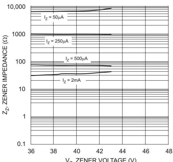
Fig. 15 Typical Zener Impedance Characteristics,
