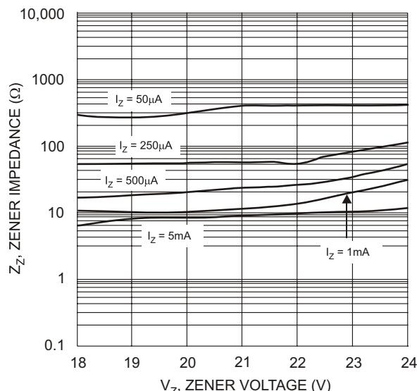
Fig. 13 Typical Zener Impedance Characteristics,
