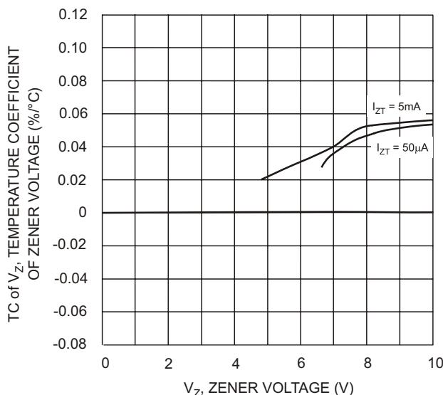
Fig. 16 Typical Temperature Coefficient of
