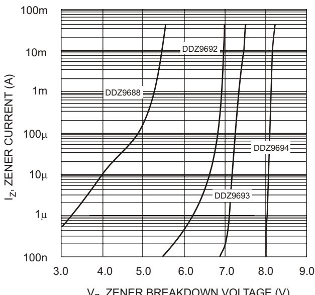
Fig. 4 Typical Reverse Characteristics, DDZ9688 - DDZ9694
