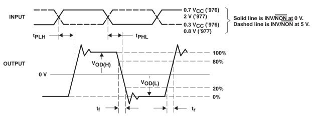
NOTES: A. All input pulses are supplied by a generator having the following characteristics:  $t_f$  or  $t_f \le 1$  ns, pulse repetition rate (PRR) = 10 Mpps, pulsewidth = 50 ns  $\pm 5$  ns,  $Z_0 = 50 \ \Omega$ .
