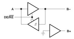
Figure 7. Noninverting Single-Ended Transceiver
