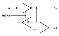
Figure 2. Inverting Single-Ended Transceiver
