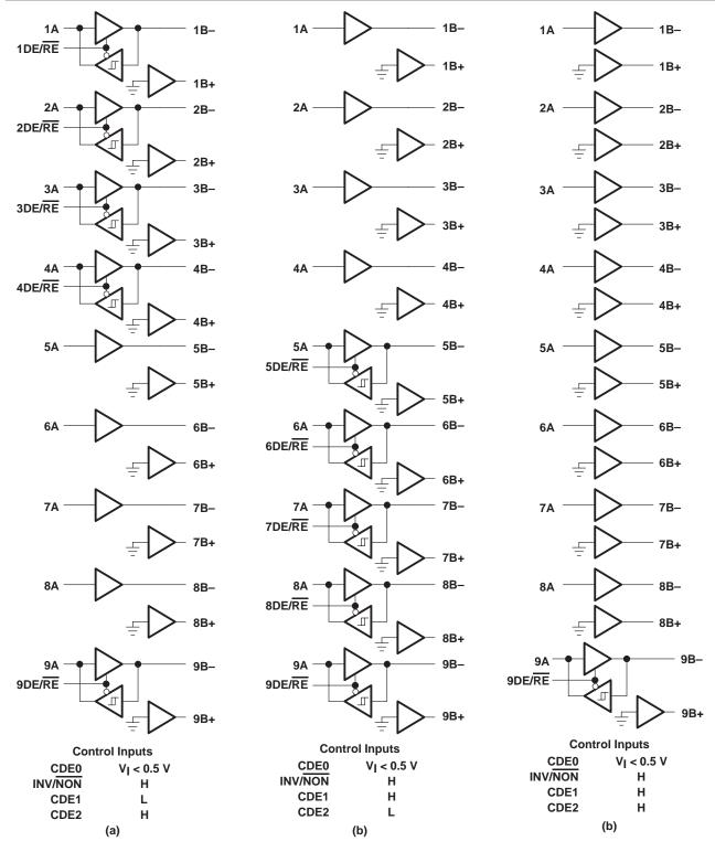
Figure 13. Logic Diagrams
