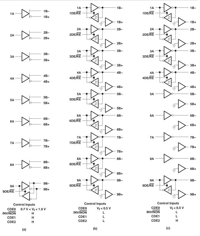
Figure 11. Logic Diagrams
