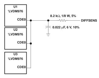
Figure 23. Low-Pass Filter for Connecting DIFFSENS to CDE0
