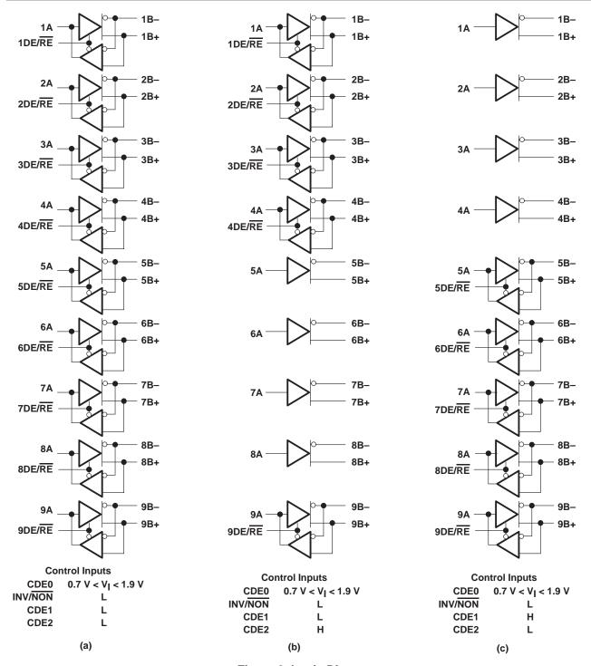
Figure 9. Logic Diagrams
