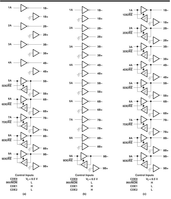
Figure 12. Logic Diagrams
