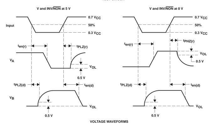
NOTES: A. All input pulses are supplied by a generator having the following characteristics:  $t_{\Gamma}$  or  $t_{\Gamma} \le 1$  ns, pulse repetition rate (PRR) = 1 Mpps, pulsewidth = 500 ns  $\pm 50$  ns,  $Z_{O} = 50$   $\Omega$ .
