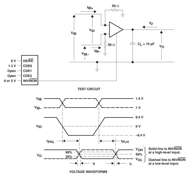
NOTES: A. Note: All input pulses are supplied by a generator having the following characteristics:  $t_{\Gamma}$  or  $t_{f} \leq 1$  ns, pulse repetition rate (PRR) = 10 Mpps, pulsewidth = 50 ns  $\pm 5$  ns,  $Z_{O} = 50$   $\Omega$ .
