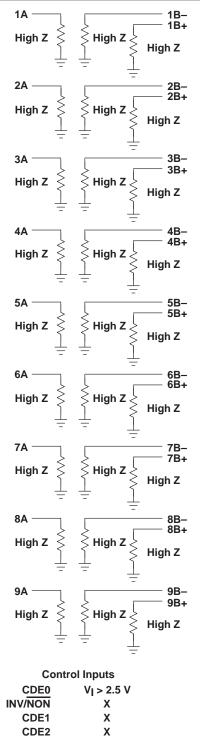
Figure 14. Logic Diagrams
