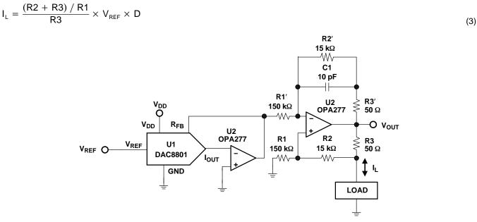
Figure 23. Programmable Bidirectional Current Source Circuit
