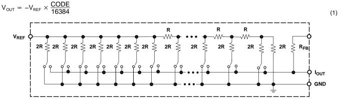
Figure 17. Equivalent R-2R DAC Circuit
