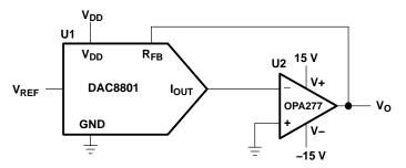
Figure 18. Voltage Output Configuration
