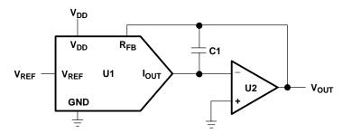
Figure 20. Gain Peaking Prevention Circuit With Compensation Capacitor
