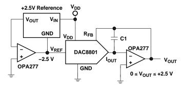
Figure 21. Positive Voltage Output Circuit
