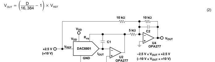
Figure 22. Bipolar Output Circuit
