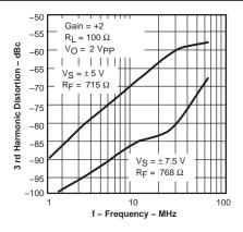
Figure 59. 3rd Harmonic Distortion vs Frequency
