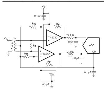
Figure 55. Differential ADC Driver Circuit 2
