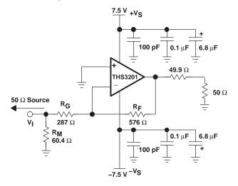
Figure 51. Wideband, Inverting Gain Configuration
