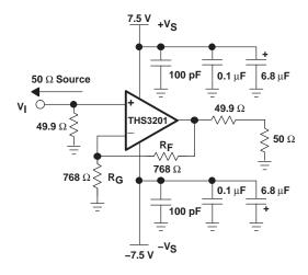
Figure 50. Wideband, Noninverting Gain Configuration
