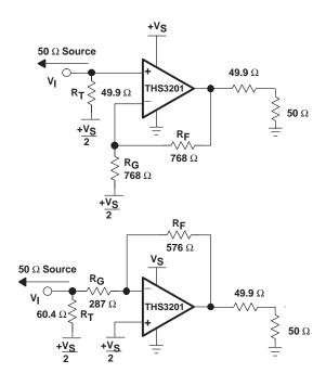
Figure 52. DC-Coupled Single Supply Operation
