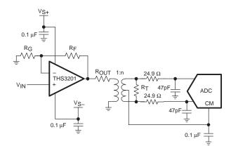
Figure 54. Differential ADC Driver Circuit 1
