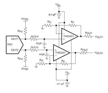
Figure 56. Differential DAC Driver Circuit
