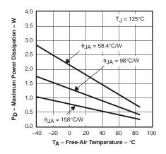
Results are With No Air Flow and PCB Size = 3"x3"  $\theta_{JA} = 58.4$ °C/W for 8-Pin MSOP w/PowerPad (DGN)  $\theta_{JA} = 98$ °C/W for 8-Pin SOIC High Test PCB (D)  $\theta_{JA} = 158$ °C/W for 8-Pin MSOP w/PowerPad w/o Solder
