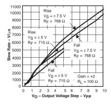
Figure 57. Slew Rate vs Output Voltage Step
