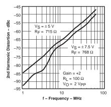
Figure 58. 2nd Harmonic Distortion vs Frequency
