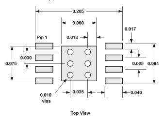
Figure 62. DGN PowerPAD PCB Etch and Via Pattern
