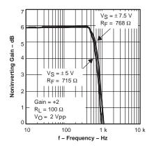
Figure 60. Noninverting Small Signal Frequency Response
