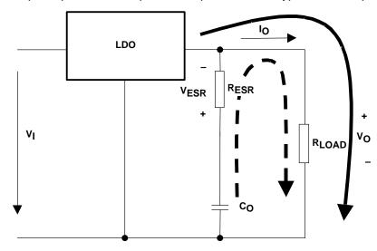
Figure 22. LDO Output Stage With Parasitic Resistances ESR
