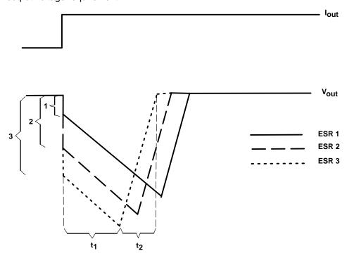
Figure 23. Correlation of Different ESRs and Their Influence to the Regulation of V<sub>out</sub> at a Load Step From Low-to-High Output Current
