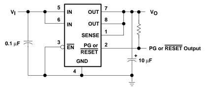
Figure 1. Typical Application Configuration (For Fixed Output Options)
