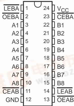
SN54LVTH543 . . . JT OR W PACKAGE SN74LVTH543 . . . DB, DGV, DW, NS, OR PW PACKAGE (TOP VIEW)
