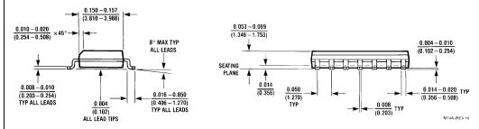
14-Lead Small Outline Integrated Circuit (SOIC), JEDEC MS-012, 0.150 Narrow Package Number M14A
