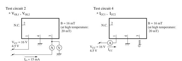
Note) \*: Measure the magnetic flux density when its output level is changed from high to low or low to high by varying the applied magnetic flux density.
